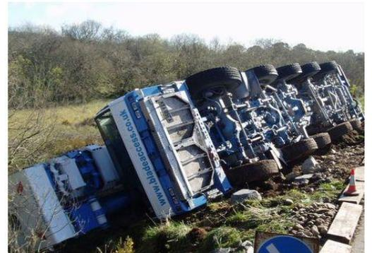
Blade's WT1000 was heading to the Gordonbush wind farm when the verge of the road gave way
